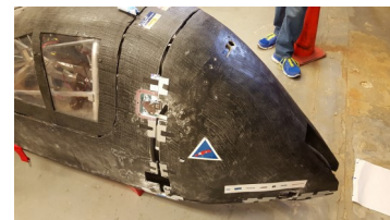
New back hatch for access to back wheel
